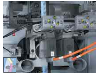
Rough trimming unit For rough trimming of all common softening materials.
